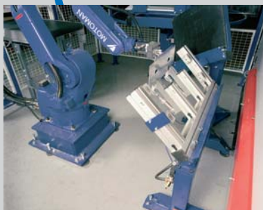
4. The regrip station, in front of the press, is used when the robot needs to change its grip between different bends.
