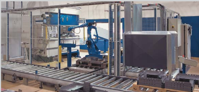
The large conveyor has room for six filled Euro-pallets without collar. Infeed magazine for 15 empty pallets.
