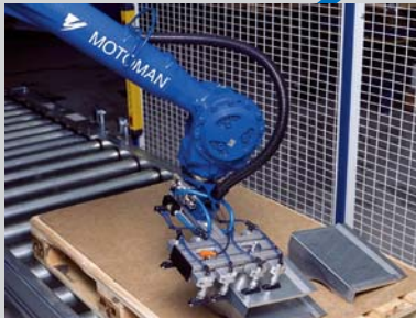
5. When the bending is complete, the robot places the finished workpieces in a desired pattern on a pallet or conveyor.
