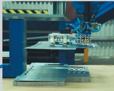
1. The robot picks up a sheet from the in-pallet or sheet magazine.
