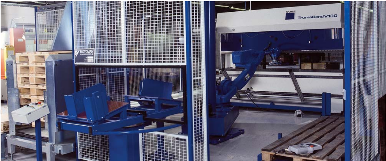
The rotating sheet magazine has two stations and can be loaded while the cell is in operation.
