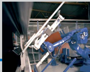
3. The robot takes the workpiece to the press and the bending sequence starts.
