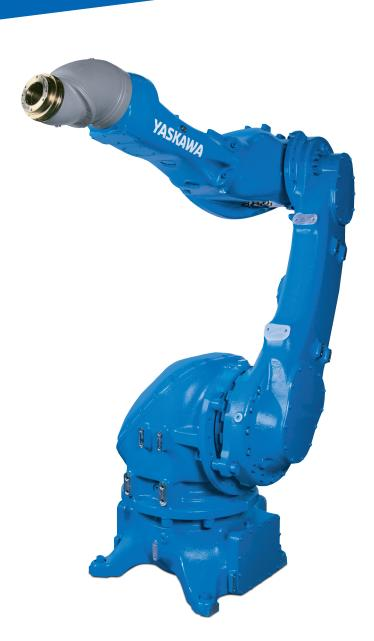
The MOTOMAN MPX2600 painting robot provides a payload of 15 kg, which enables mounting of multiple guns and large bells on this medium-sized robot. The smooth arm design with a large hollow diameter is optimal for tubing and can prevent interferences among paint and air tubes. On the U-Arm additionally paint equipment can be mounted.
