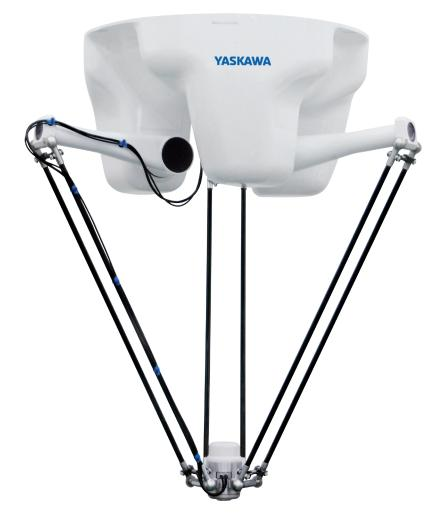
The MOTOMAN MPP3H 4-axis high-speed robot with parallel kinematic system combines the speed of the delta design with a high payload capacity and a large working range. Due to the high torque of the fourth axis, the so-called wrist axis, the MOTOMAN MPP3H moves payloads of up to 3 kg at unprecedented speeds. This delta robot was developed for a wide spectrum of industries, such as food and beverage, pharmaceutical and the automotive sector.
